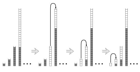
Figure 1. Making room for one new element in a multistack.
